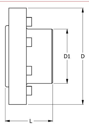
D = 315 D1 = 200 L = 140 Max bore = 120 Torque (N m) = 5500
